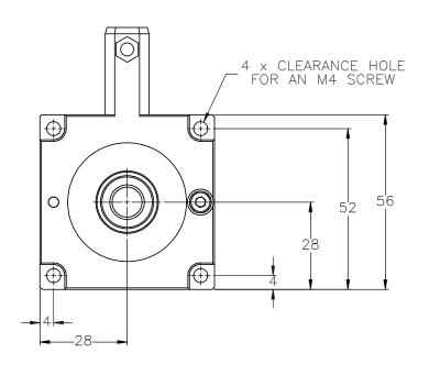
ACTUATOR BODY T-SLOT MOUNTING FEATURES
