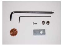
The tools and parts you will need include a M2 and a M4 wrench, a penny, an M3x10 bolt, the M8x8 and M8x6 set screws, and a sensor T-Nut.
