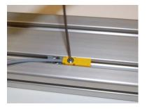
Place the sensor down with the wire running towards the drive shaft, and tighten with the M2 wrench.
